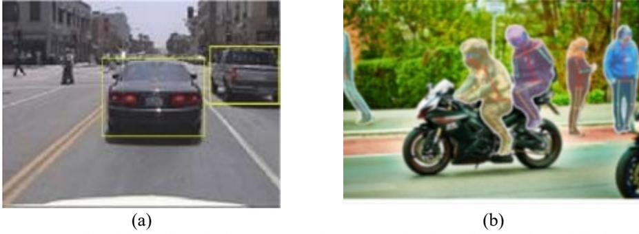
Figure 11. Examples of object detection by (a) YOLOv4 in a rectangular shape (from mathworkk [24]) and (b) Mask R-CNN (courtesy of He et. al [22])
