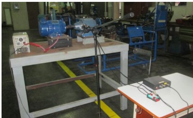
Figure 1. Microphone and transmitter are installed on a gearbox transmission
