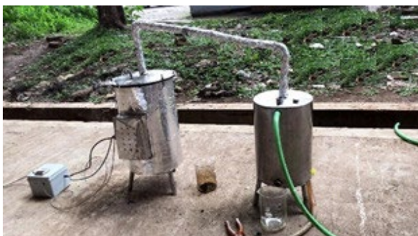
Figure 2. The Design of Pyrolysis Reactor
