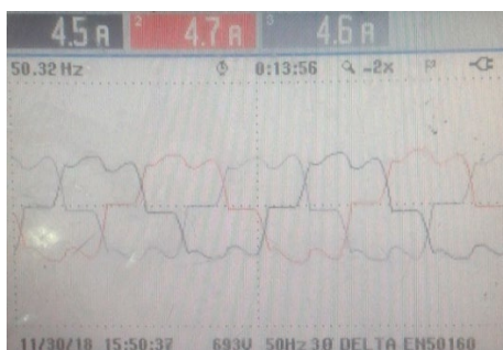
Figure 2. Voltage and current waveforms at the generator load by the DC motor with a VSD
