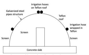
Figure 1. Architectural Configuration of Screen House
