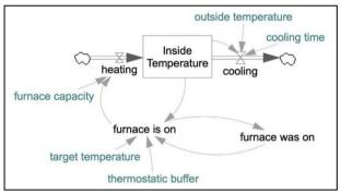
Figure 2. The System Design Model in Vensim Software
