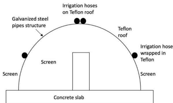
Figure 1. Architectural Configuration of Screen House
