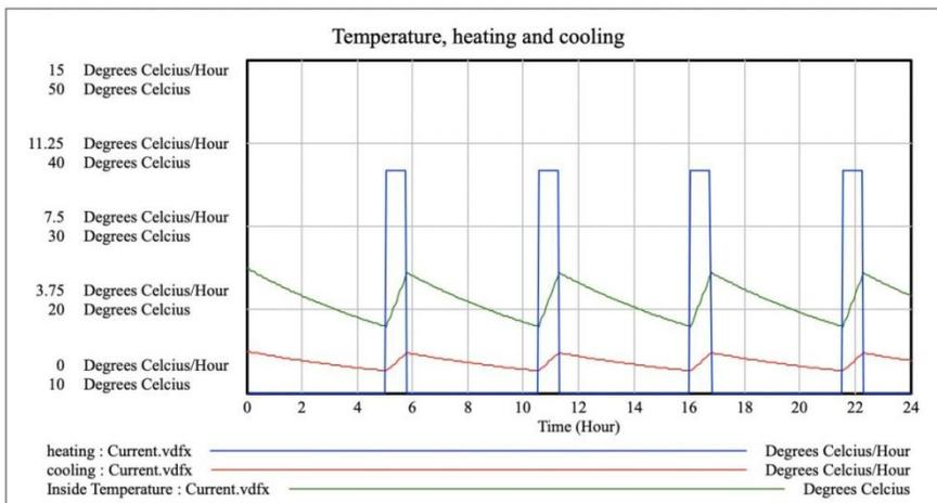
Figure 3. The Simulation Result of Screen House Microclimate Conditioning System
