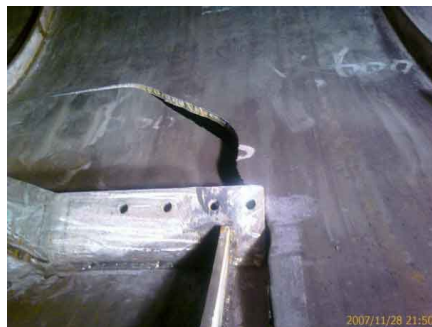
Figure 1. Crack occurs in a pressure vessel during hydro test (Source: www.wermac.org )
